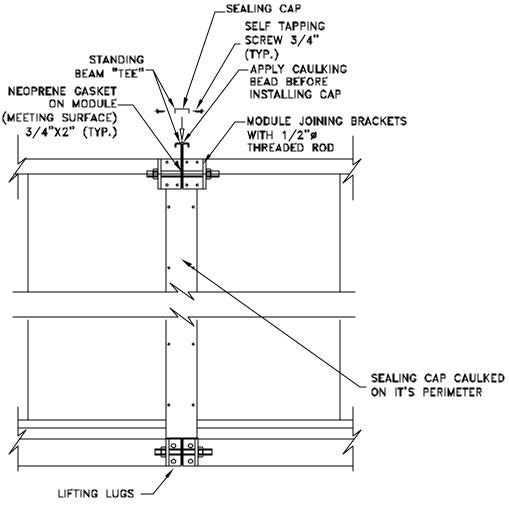
NOTE: DO NOT USE LIFTING LUGS & BOLTS TO BRING MODULE TOGETHER
