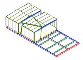
5. Use a ratchet hoist to pull the second module to the first module
