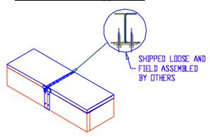
9. Install factory supplied exterior side cap over center of seam and screw in place with factory provided screws. Caulk along the perimeter of exterior cap with factory supplied caulking.
